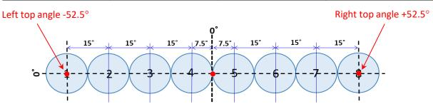
4.20 Mechanically tilt the antenna toward the target area and secure it firmly.
