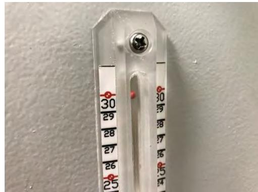
During calibration, the RET Element will use an Upper & Lower hard-stop to calibrate 0 - 30 Degree range. All 12 Beams / RET Elements offer a tilt rang from 0 to 30 degrees independantly. The current degree of tilt is indicated by the movable red marker tip.
