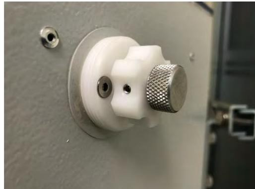
Step 2) Unscrew the metal locking stub.
