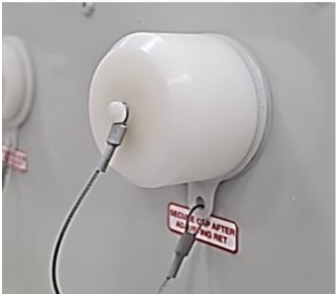
Engaged with internal RET motor position
