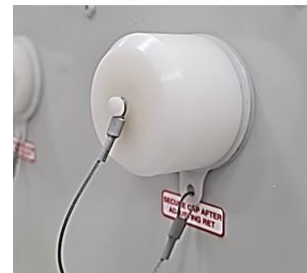
Unscrew/Screw the cap for tilt adjustment process
