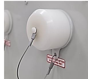
Unscrew/Screw the cap for tilt adjustment process
