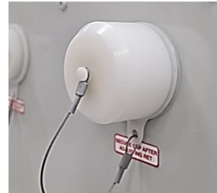
Unscrew/Screw the cap for tilt adjustment process
