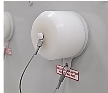
Unscrew/Screw the cap for tilt adjustment process
