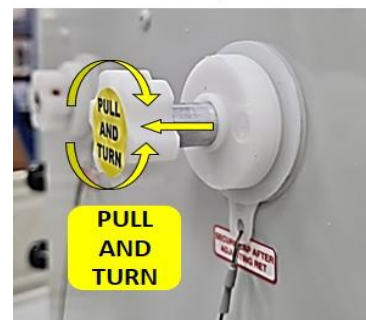
Pull handle out to disengaged RET for tilt adjustment
