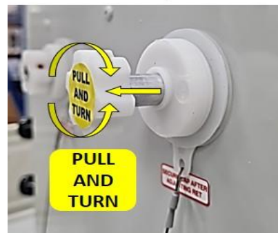
Pull handle out to disengaged RET for tilt adjustment
