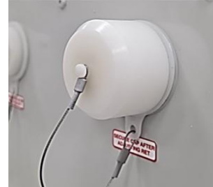
Unscrew/Screw the cap for tilt adjustment process
