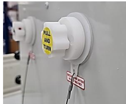
Engaged with internal RET motor position
