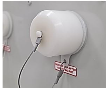
Unscrew/Screw the cap for tilt adjustment process
