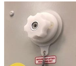
2. Unscrew/ Screw the cap for tilt adjustment process
