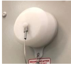
1. Engaged with internal RET motor position
