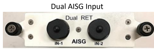
IN-1 Controls LB Beams 1
