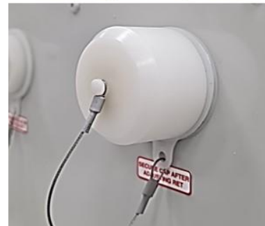
Unscrew/Screw the cap for tilt adjustment process
