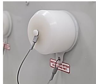
Unscrew/Screw the cap for tilt adjustment process
