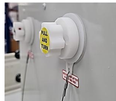
Engaged with internal RET motor position
