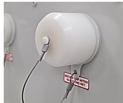
Unscrew/Screw the cap for tilt adjustment process
