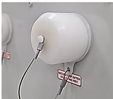
Unscrew/Screw the cap for tilt adjustment process
