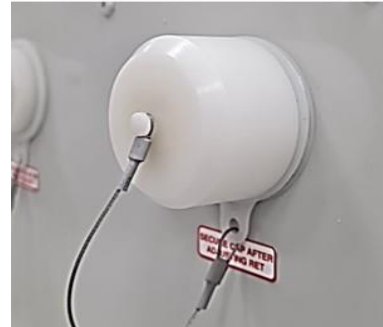
Unscrew/Screw the cap for tilt adjustment process
