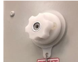
Unscrew/Screw the cap for tilt adjustment process
