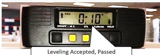
ANTENNA LEVELING ACCEPTED
