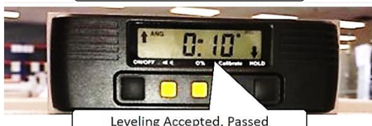
ANTENNA LEVELING ACCEPTED
