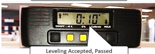
ANTENNA LEVELING ACCEPTED
