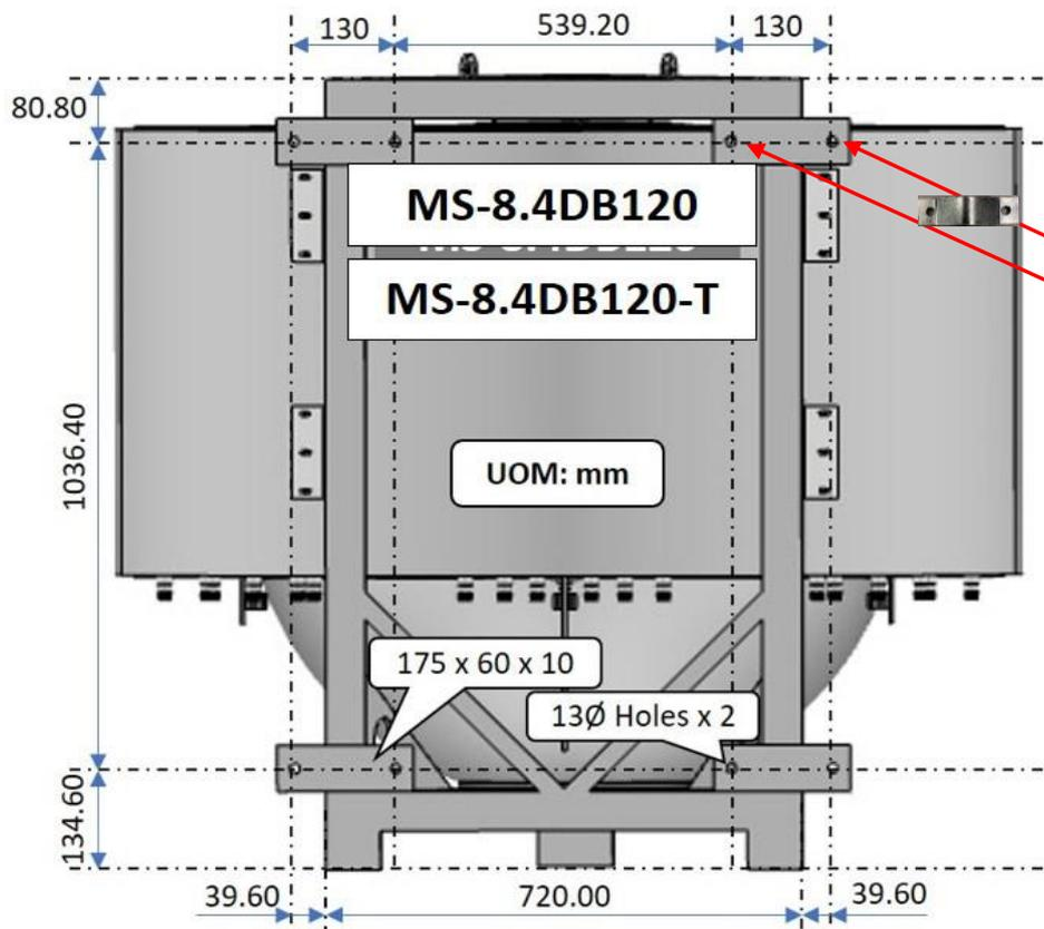
Tighten to the pole with Bolt & Nuts Sets
