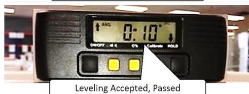
ANTENNA LEVELING ACCEPTED
