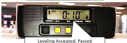
ANTENNA LEVELING ACCEPTED
