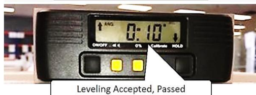
ANTENNA LEVELING ACCEPTED
