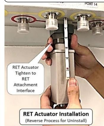
Step 7: Screw and tighten RET cable
