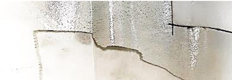
Sample 2: Glass Fabric Detached & Tear
