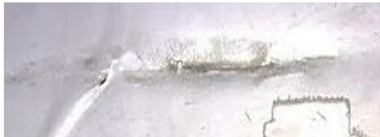
Sample 4: Glass Fabric & Styrofoam Dented
