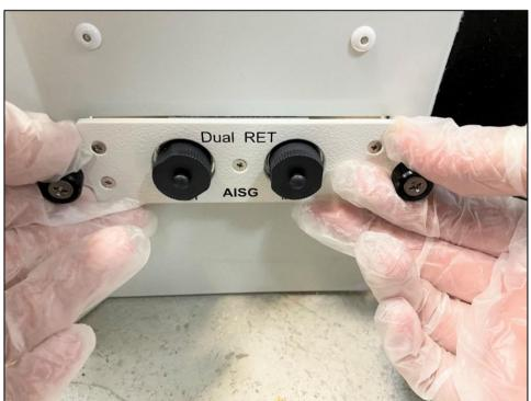
1.03 Replace with a new controller. Ensure the controller SN# tally with Antenna SN#
